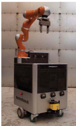
Fig. 1. Little Helper 3, an AIMM at Aalborg University designed for attending complex assembly tasks.
