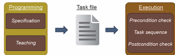
Fig. 4. Illustration of the correlation between the programming part and the execution part of a task. During the programming part the sequence of skills is established and a set of parameters is obtained through a programming routine. This information is stored in a task file, from which the task can later be executed. The programming part is divided into a specification phase and a teaching phase.
