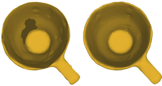
Fig. 17 3D models of coffee cup from top with standard ICP registration ( left ) and extension by considering normals ( right ).
