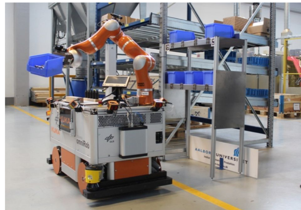
Figure 2: The omniRob carrying out part logistics, transporting finished assembled goods from the assembly station to the warehouse.
